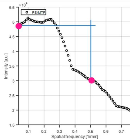
Figure 4: PS/MTF curve for image section from figure 3
