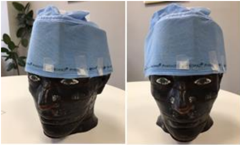
Figure 15: Position of the TLDs placed on the lead-free cap used in hospital A during the second phase.
