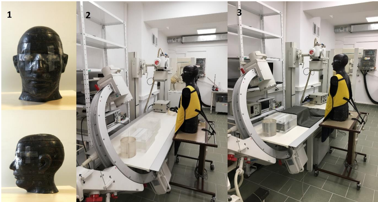
Figure 20: Measurement of the efficiency of a lead drape (LITE TECH, INC., USA) on a RA phantom in a clinical set-up: 1) position of dosimeters on the left temple and the eye lens, 2) LAO 30 projection without the lead drape, 3). LAO 30 projection with the lead drape.
