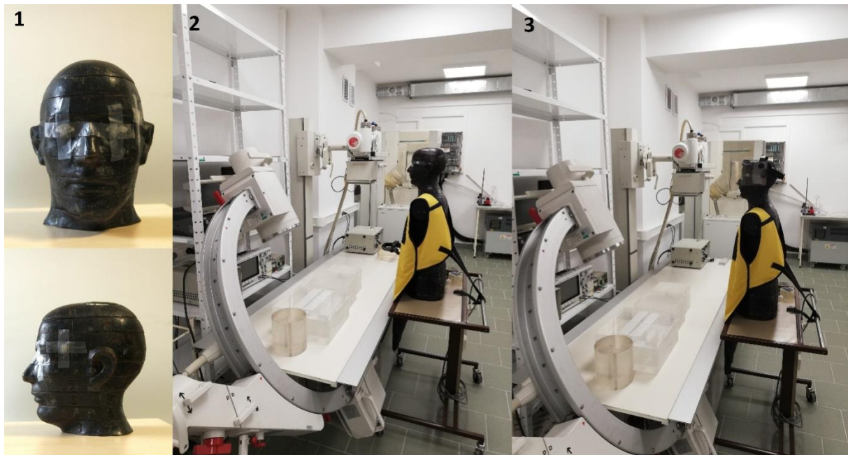
Figure 19: Measurement of the efficiency of a mask (model M1) on a RA phantom in a clinical set-up: 1) position of dosimeters on the left temple and the eye lens, 2) LAO 30 projection without the mask, 3).LAO 30 projection with the mask.
