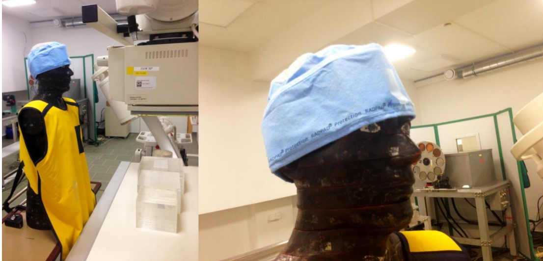
Figure 18: Measurement of the efficiency of a lead-free cap on a RA phantom in a clinical set-up (LAO 30 projection).
