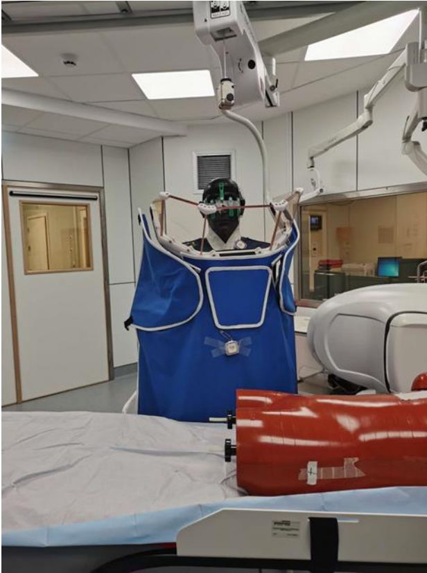
Figure 21: Measurement of the efficiency of the ZG system on a RA phantom in a clinical set-up.
