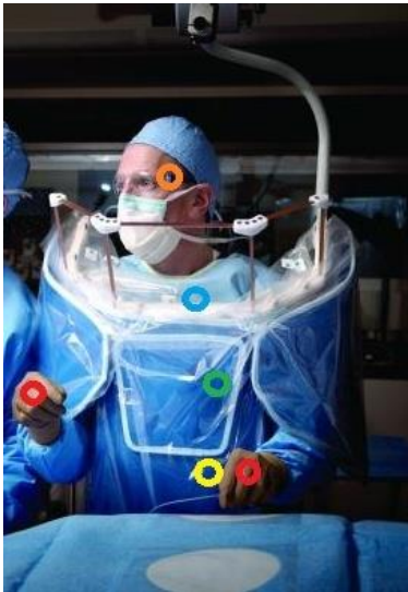
Figure 17: Position of the dosimeters in hospital J for assessment of the ZG suspended system efficiency
