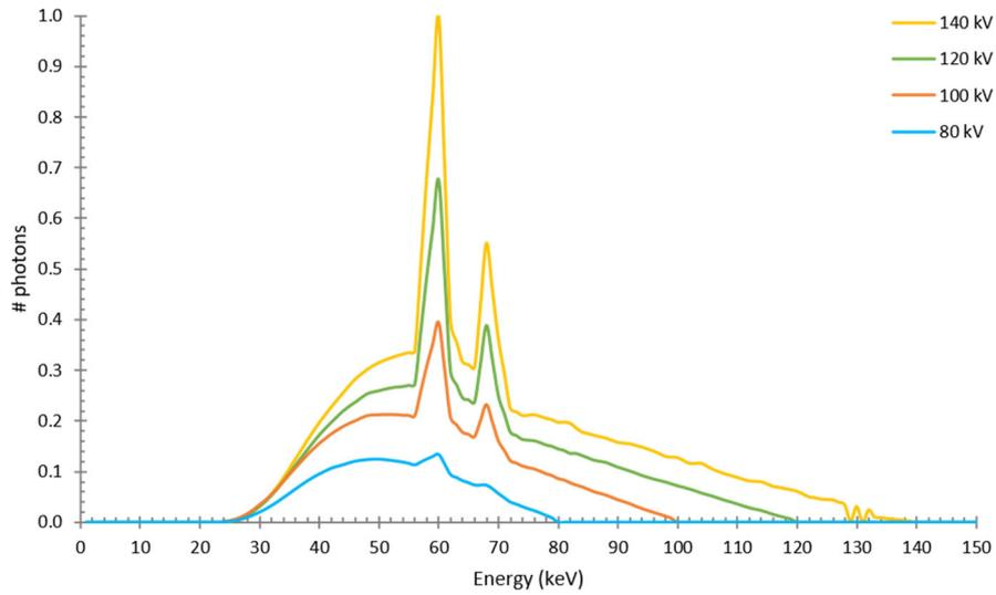
Figure 10: Normalised equivalent X-ray spectra based on half-value layer measurements and generated with a voltage ripple of 0%.
