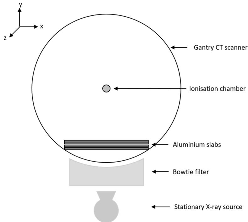
Figure 9: Set-up of half-value layer measurement (based on [16]). In case CT exposure cannot occur without the CT table in the X-ray beam path, the X-ray source and aluminium slabs are positioned laterally at the 3 o'clock position.
