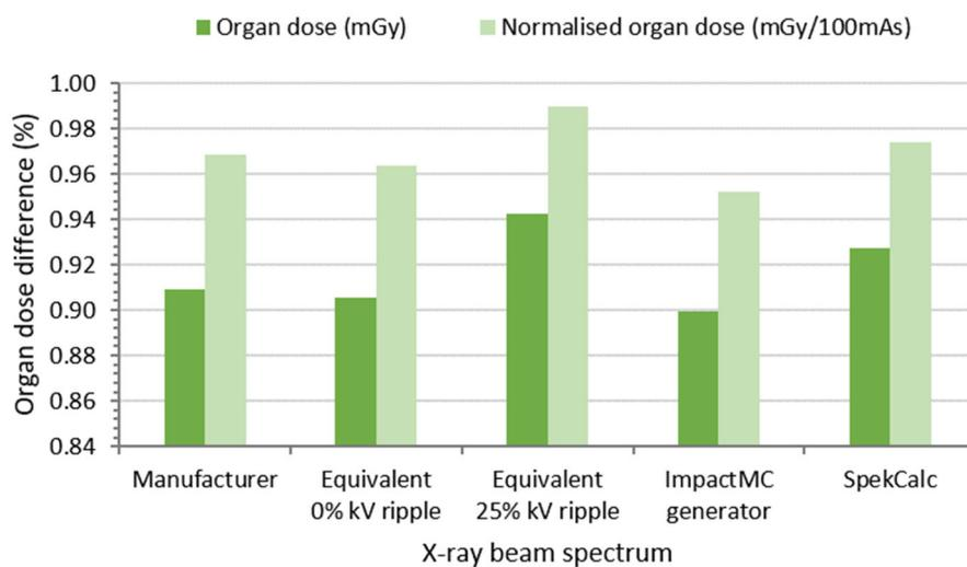
Figure 13: Maximum percentage difference in mean organ dose between the two bowtie models used for the Monte Carlo simulation of a diagnostic whole-body CT scan in hybrid imaging. Note that the assumption was made that the bowtie filter model provided by the manufacturer is the real filter model.
