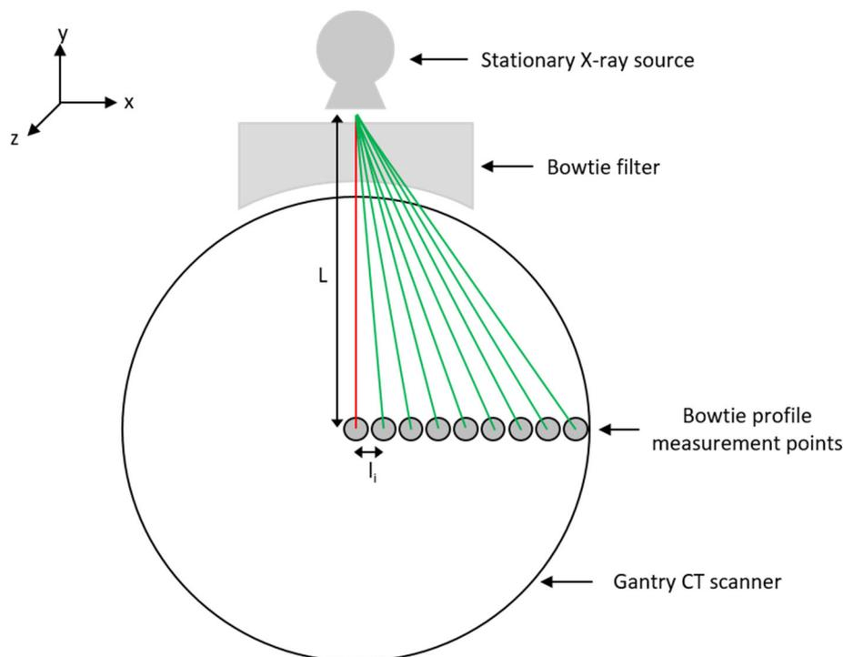
Figure 3: Set-up of CT bowtie profile dose measurements, with  $L$  the focus to isocenter distance and  $l_i$  the distance between the measurement points (figure based on [16]).
