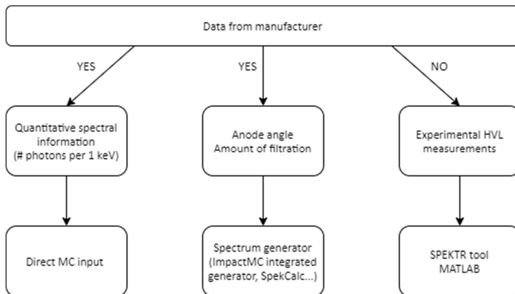
Figure 2: Schematic overview of different possibilities to obtain X-ray beam spectrum for each tube voltage.
