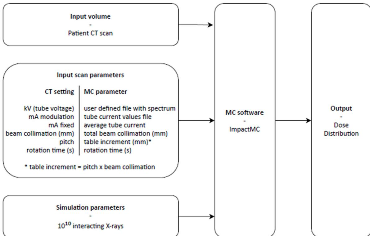
Figure 4: Overview of the input needed for Monte Carlo (MC) dose calculations with ImpactMC and the resulting output.
