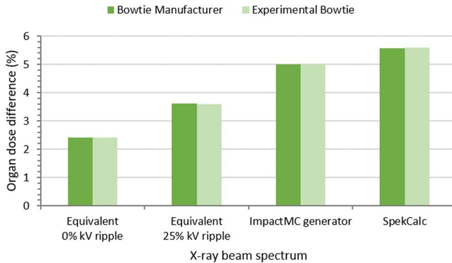
Figure 14: Maximum percentage difference in mean organ dose for the different X-ray spectra used for the Monte Carlo simulation of a diagnostic whole-body CT scan in hybrid imaging compared to simulations using the spectrum provided by the manufacturer. Note that the assumption was made that the X-ray spectrum provided by the manufacturer is the real spectrum. Results are given for simulations performed with the bowtie model from the manufacturer and experimental dose measurements, respectively.
