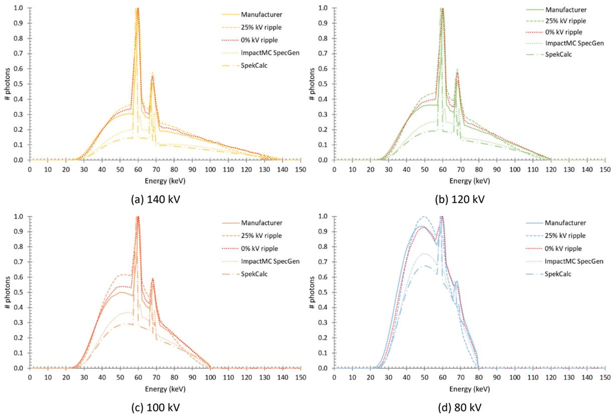
Figure 11: Graphical comparison of the (a) 140 kV, (b) 120 kV, (c) 100 kV and (d) 80 kV X-ray spectra provided by the manufacturer, created with the SPEKTR tool applying a 25% and 0% voltage ripple after half-value layer measurements, and generated with the ImpactMC integrated spectrum generator and SpekCalc.
